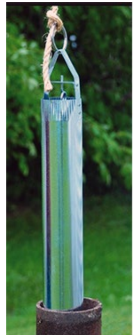
The well bucket attached by a rope through the pulley is lowered into the well. A flap at the bottom allows water in. When raised, the ring at the top is pulled to release the water.
